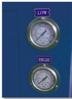
● High and low pressure of hydraulic chuck.
